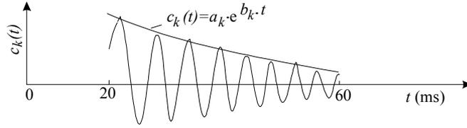
Figure 2: Acceleration of the specimen - average signal (schematically).
