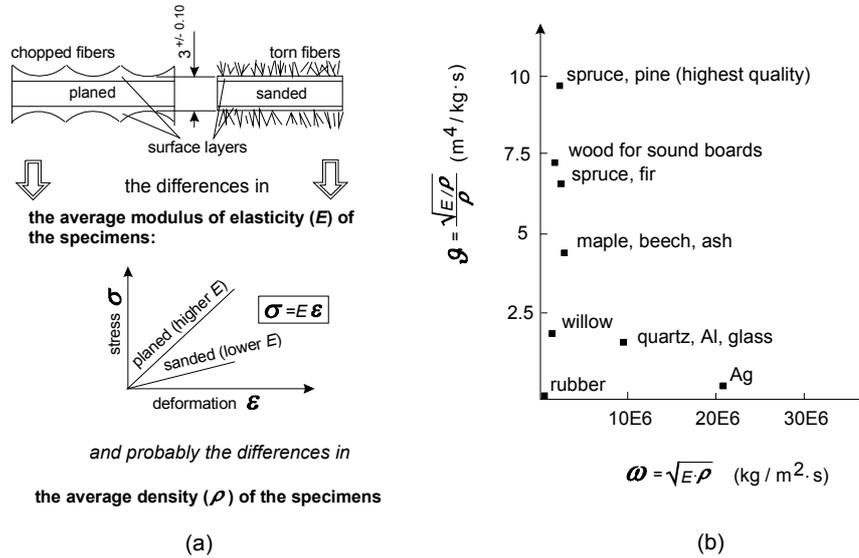
Figure 4: Relation between acoustic and mechanical properties: (a) the mechanical consequence of the different surfaces of planed and sanded specimens; (b) dependence of the damping of sound radiation on the sound wave resistance for different wood species and other materials.  $\omega$  and  $\mathcal{G}$  were obtained from Kollmann & Côté (1968).
