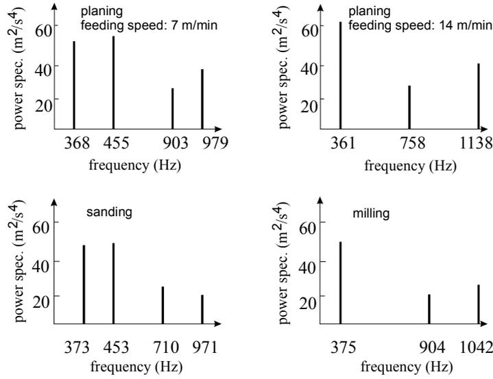
Figure 3: Spectral characteristics of the acceleration (wood B).
