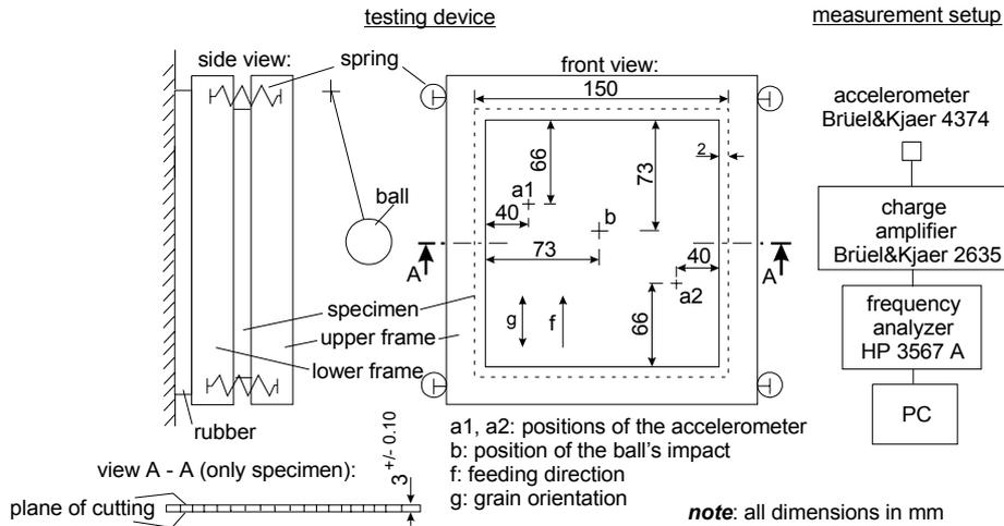
Figure 1: Testing device, specimen orientation and measurement set-up.
